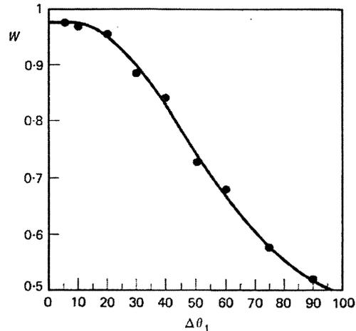
Figure 3. Normalized autocorrelation  $W$  measured for several values of  $\Delta\theta_1$ , for a surface roughness  $R_a = 3.2 \mu\text{m}$ .
