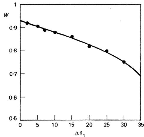
Figure 5. Normalized autocorrelation  $W$  measured for several values of  $\Delta\theta_1$ , for a surface roughness  $R_a = 25 \mu\text{m}$ .
