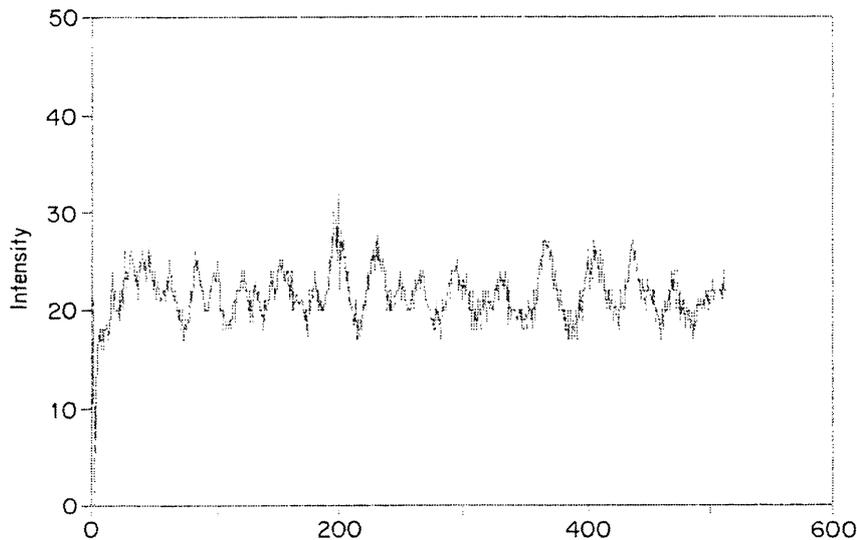
Figure 2. Intensity distribution of a recorded double speckle pattern.
