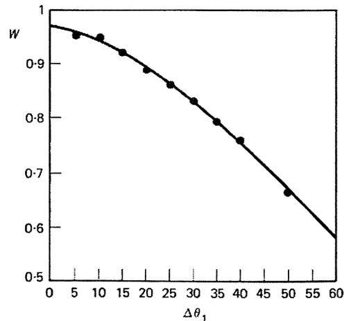
Figure 4. Normalized autocorrelation  $W$  measured for several values of  $\Delta\theta_1$ , for a surface roughness  $R_a = 6.3 \mu\text{m}$ .
